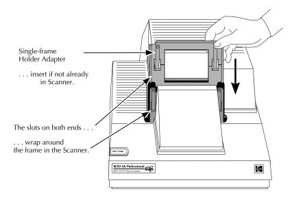
3. Place the film holder into the Scanner by sliding it down completely into place behind the single-frame holder adapter; be certain that the film holder is aligned with the indentation in the frame in the Scanner.
